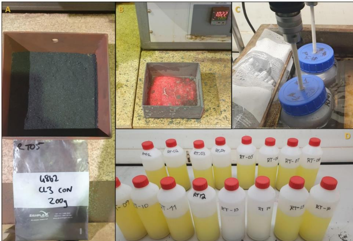
Figure 4: Photos showing A) Magnetic concentrate prior to roasting, B) Sample removed from oven after roasting, C) Water leaching from roasted sample & D) Filtered liquor containing leached Vanadium.
